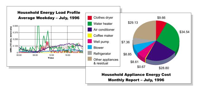
The SPEED<sup>™</sup> product line is based on Non-Intrusive Appliance Load Monitoring System (NIALMS) – technology developed initially by Telog Instruments, Inc. under the sponsorship of the Electric Power Research Institute (EPRI). SPEED products are now available after successful testing and performance verification under actual application situations at nine utilities.
